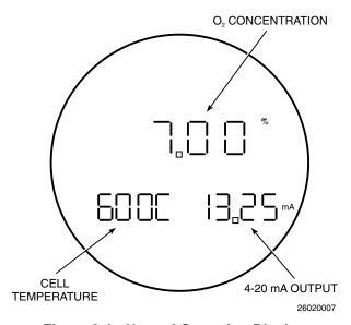
Figure 3-1. Normal Operation Display
